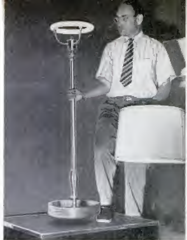
John Campbell shows that fluorescent tube of lamp glows brightly even when lamp is lifted from floor
